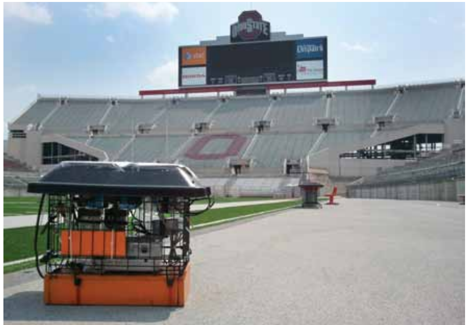
The cage, shown in Ohio Stadium, houses equipment to measure carbon monoxide, carbon dioxide, black carbon and particulate matter which are all indicators of car, bus and truck traffic. Multiple locations throughout campus were monitored for one full week.
